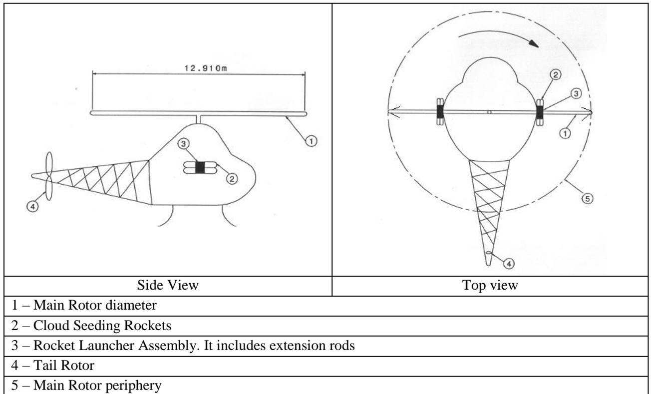
Figure 3(b): Retracted position of attachments.
