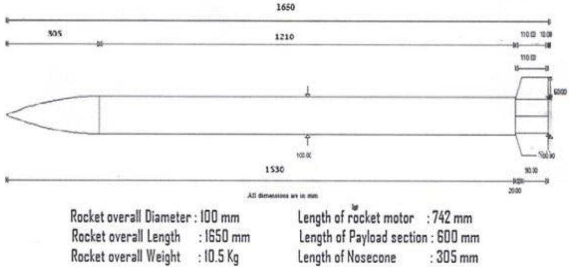
Figure 3(a): Design specification of AgI Rocket (Kumar et al. 2015).
