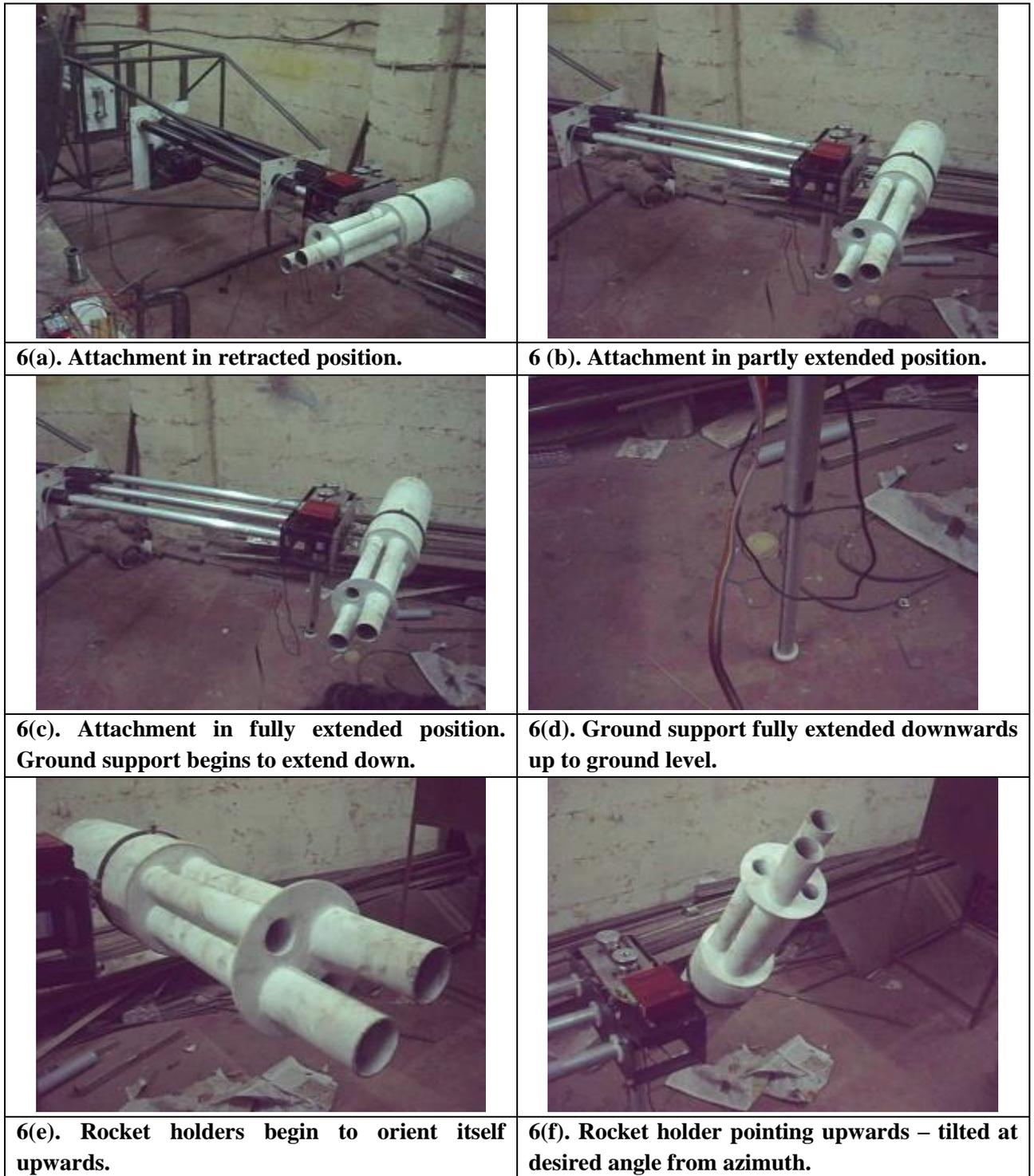
**Figure 6: Workshop fabrication of attachment on half size dummy model of Cheetah helicopter.**
