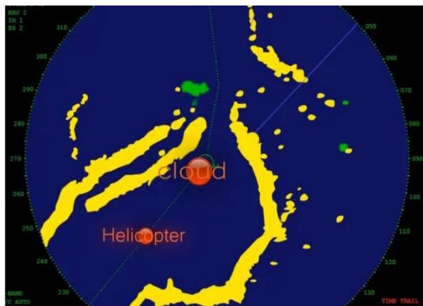
**Figure 2: Screen installed before the pilot in the cockpit displays the area map and the spots of current location of Helicopter and that of cloud.**
