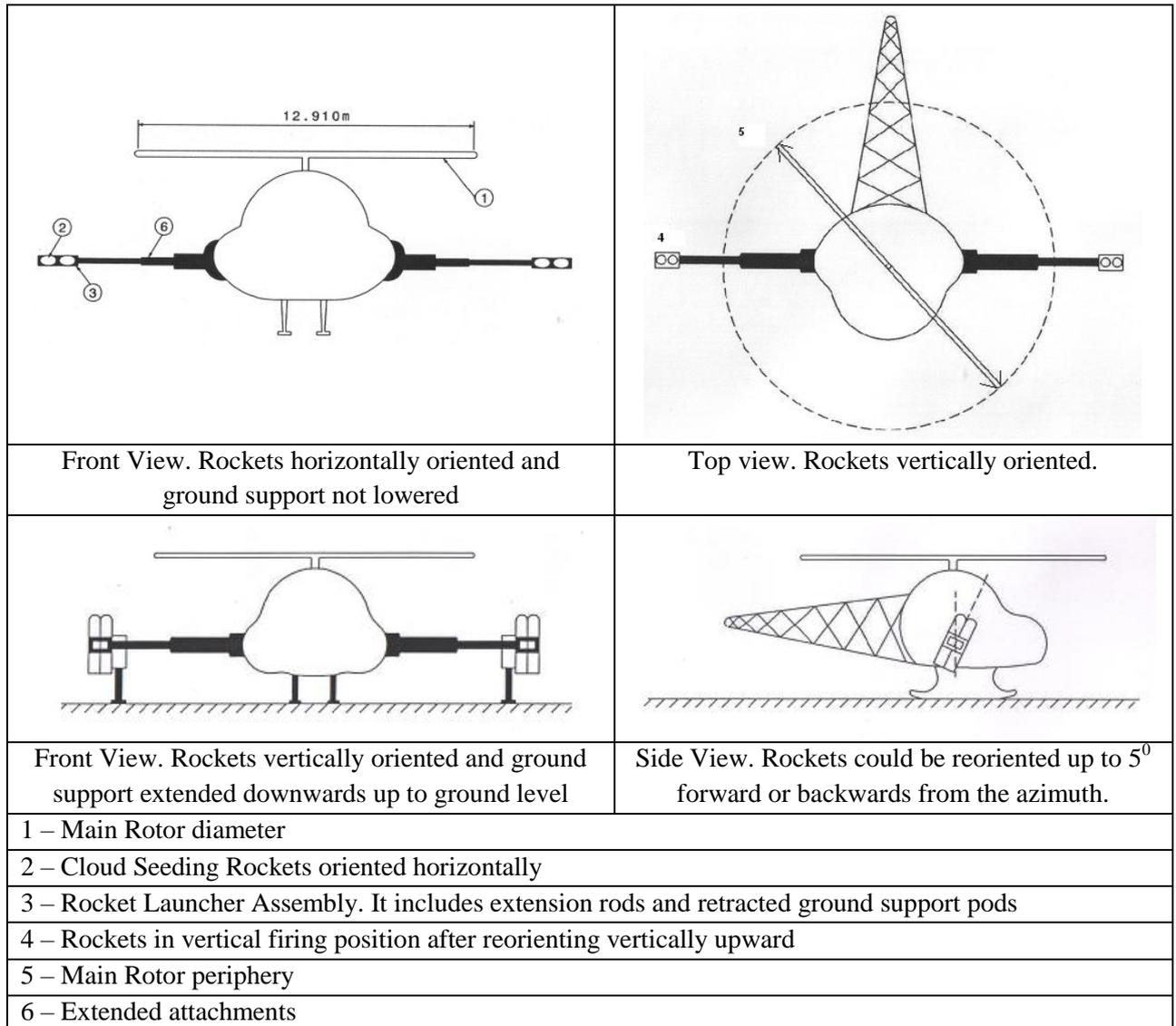
**Figure 4: Extended position of attachments.**
