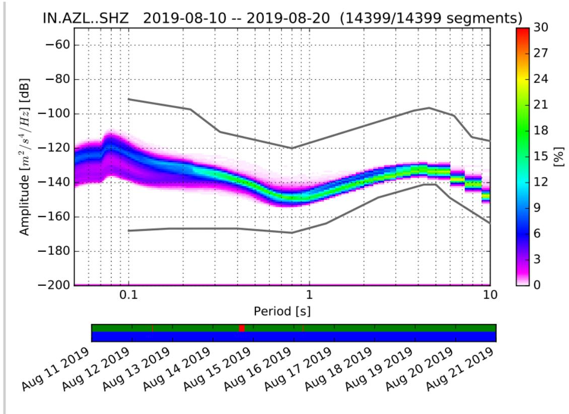
Figure 2 (c): PPSD analysis for Seismic Station at AIZAWAL (AZL) (11-21 August-2019)
