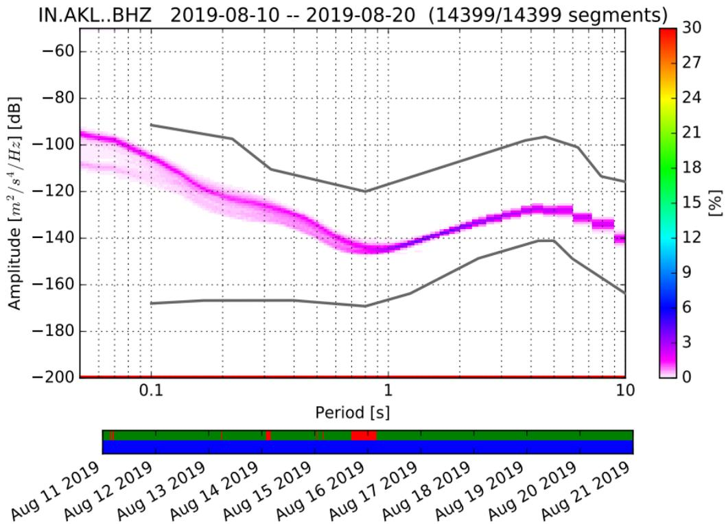
Figure 2 (b): PPSD analysis for Seismic Station at AKOLA (AKL) (11-21 August-2019)
