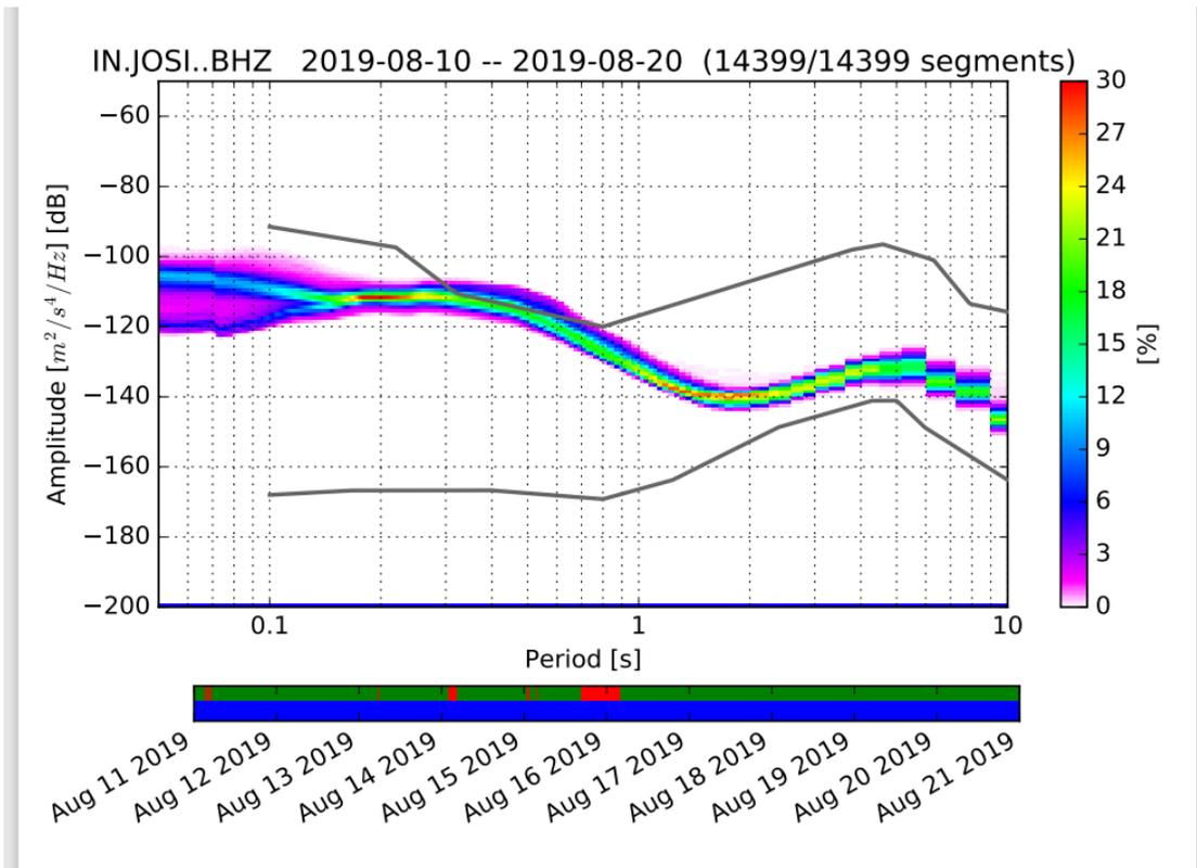
Figure 2 (e): PPSD analysis for Seismic Station at JOSIMATH (JOSI) (11-21 August-2019).
