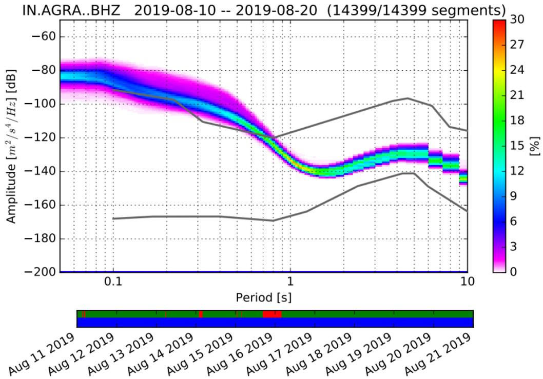
Figure 2 (a): PPSD analysis for Seismic Station at Agra (11-21 August-2019).
