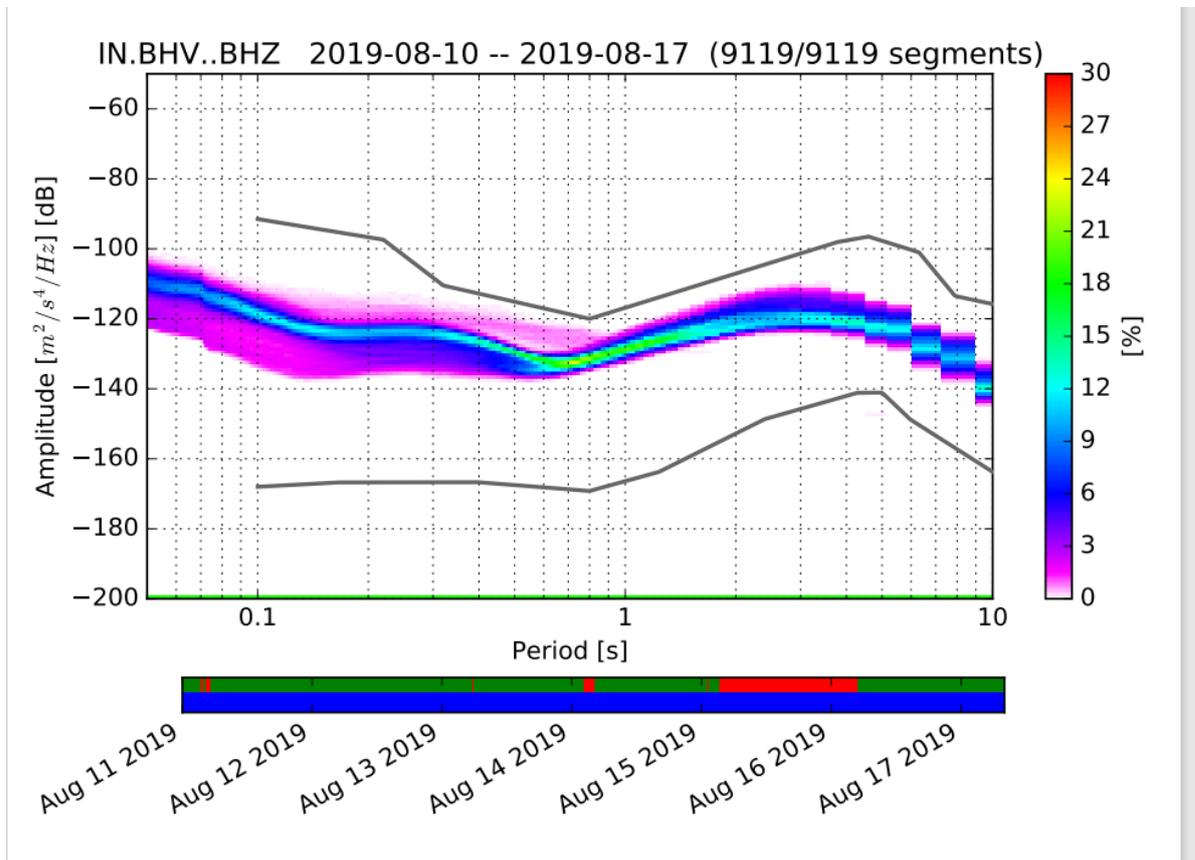
Figure 2 (d): PPSD analysis for Seismic Station at BHAVNAGAR (BHV) (11-17 August-2019).
