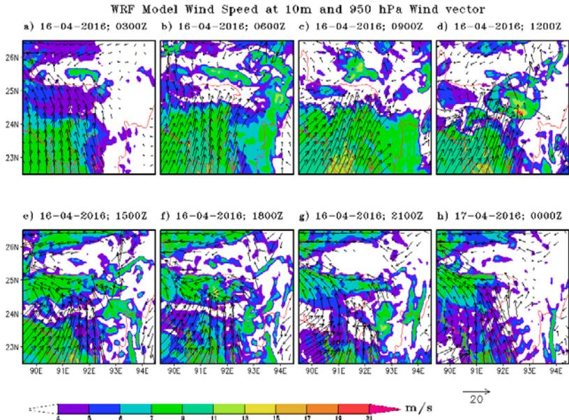
Figure 3: WRF model simulated forecasted vector wind at 950 hPa and wind speed at 10m
