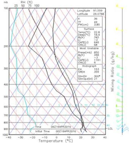
Figure 2b: skew-T simulated model at 0600 Z of 16 April 2016
