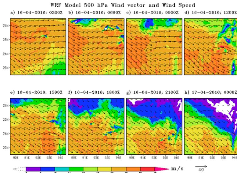
Figure 4: WRF model simulated forecasted vector wind at 500 hPa
